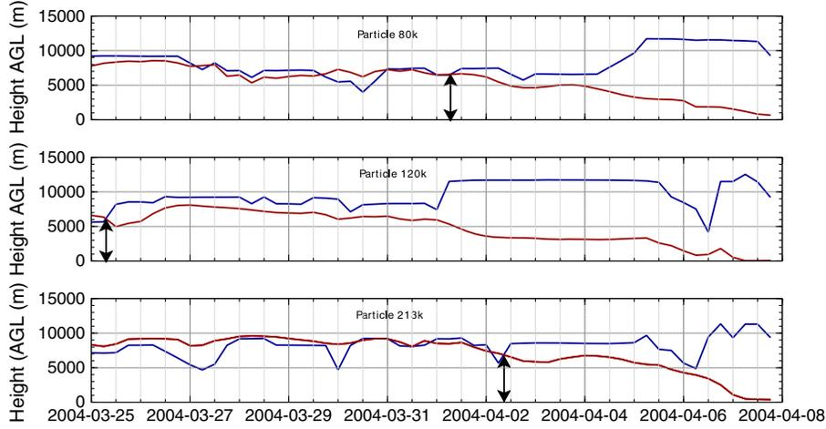
**Figure 6.** Vertical trajectories of selected particles, as a function of time, as they move toward the Harlech sampler. Sampling ends at 8 April 00 UTC. The dark red line represents the particle position, and the dark blue line represents the tropopause height (2 PVU level) at the particle position. The vertical arrows indicate the time when the particle exits the stratosphere for the last time. This defines the “exit time” used in the study.
