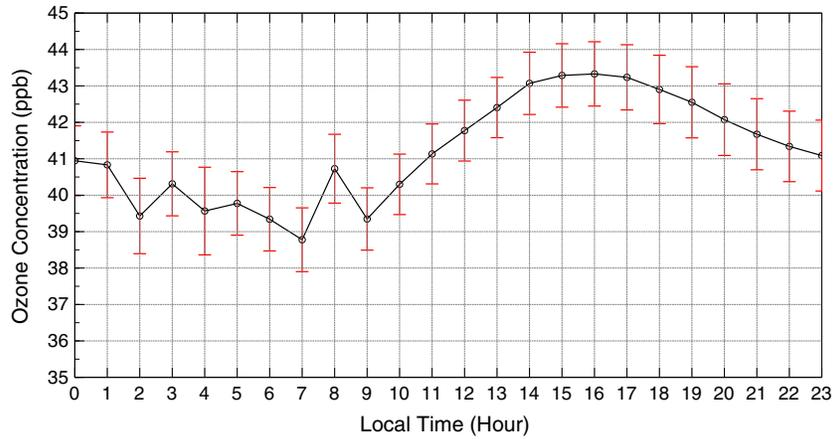
**Figure 3.** Mean diurnal variation of O<sub>3</sub> concentrations measured at Harlech for July 2003 to June 2004. The error bars represent the 95% confidence interval for each hourly mean.
