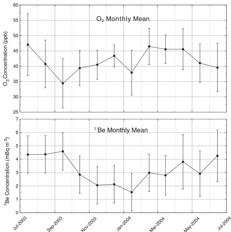
**Figure 2.** Monthly averages of <sup>7</sup>Be and O<sub>3</sub> concentrations measured at Harlech for July 2003 to June 2004. The O<sub>3</sub> error bars show the standard deviation of the daily means for each month. The <sup>7</sup>Be error bars use the standard deviation of all the weekly averages (1.39 mBq m<sup>-3</sup>) from June 2003 to February 2004, and the standard deviation of the daily means of each month for March, April, May, and June 2004.
