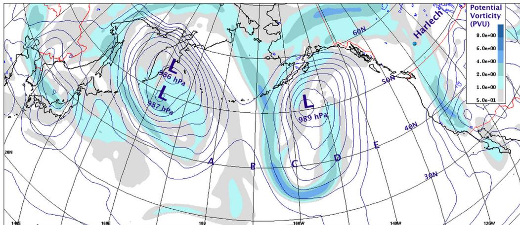
**Figure 11.** Potential vorticity (PV) 6000 m above the surface (color shading) and mean sea level pressure (continuous lines) valid 2 April 2004 00 UTC. The depth of the Pacific low pressure centers is shown in hPa, and the approximate position of the lowest pressure is indicated by a “L.” A cross-section of the 3-D PV field along latitude 40°N, from points labeled A to E is shown in Figure 12.
