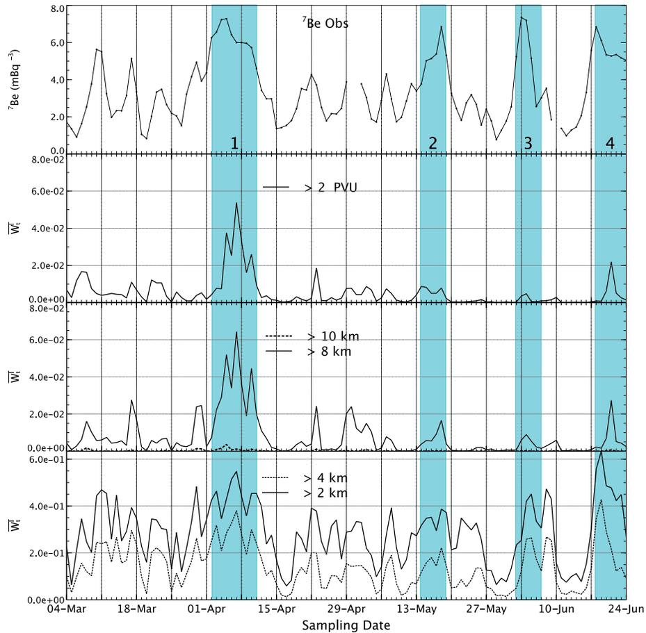
**Figure 7.** Observations of (top)  $^7\text{Be}$  daily average concentrations compared to the weighted layer residence time fraction,  $\overline{W}_t^w$ , for various layers during the period March to June 2004. Note the scale differences in the  $\overline{W}_t^w$  values on the different panels. The cyan colored areas, numbered 1 to 4, correspond to investigated events.
