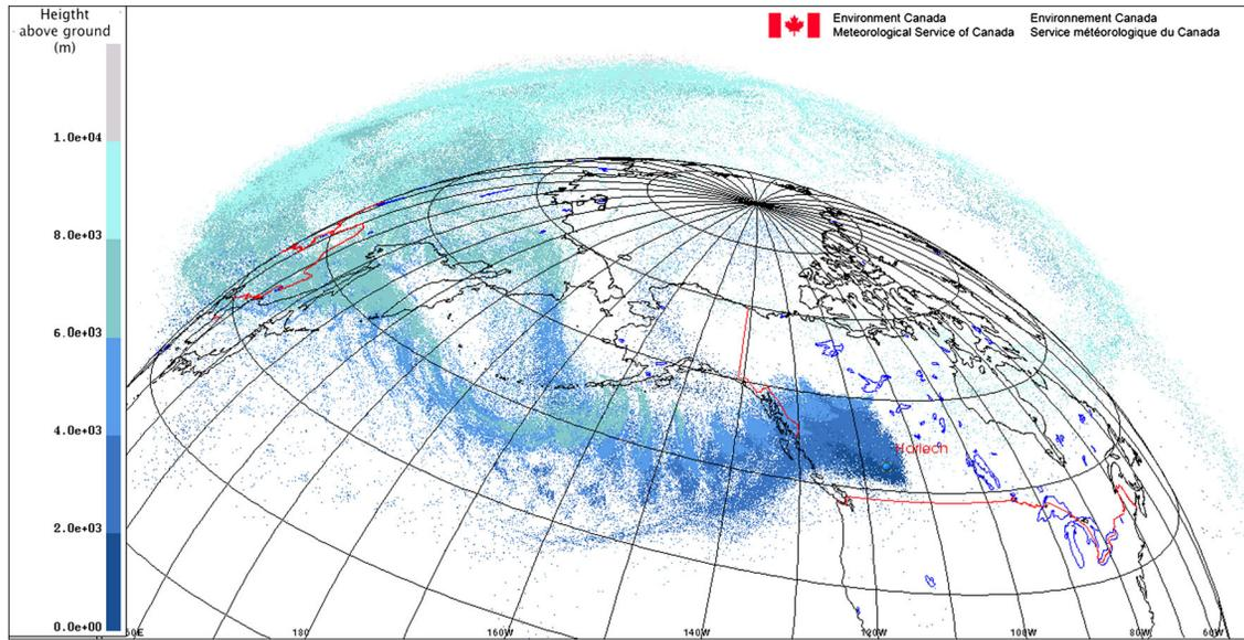
**Figure 10.** Time-integrated plume of the stratospheric particles (i.e., particles that have been above the 2 PVU level at least once), sampled at Harlech during the 24 h period ending 8 April 00 UTC. Particles were sampled from a reduced set of all the particles used in the simulation and are shown every 6 h during their 14 day trajectory toward Harlech.
