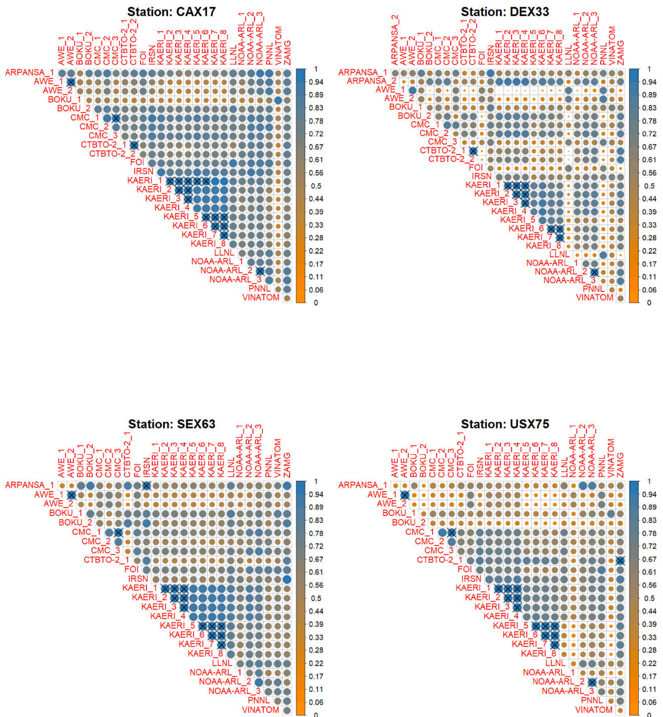
Fig. 7. Correlation matrix calculated for all model results available at the four locations for the period June to November 2014 including all samples equal to or above the MDC. The correlation of results is indicated by the color and the size of the symbol. The larger the symbol the higher the correlation. All models showing a correlation larger than or equal to 0.95 are indicated with a cross through the symbol. (For interpretation of the references to color in this figure legend, the reader is referred to the Web version of this article.)
